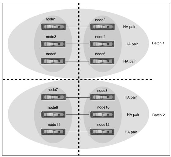
**Note:** The node names in this diagram are provided for example purposes only. The nodes are numbered to depict the proper upgrade sequence.
